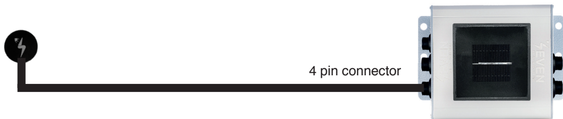
Figure 11 – Connection of the 3S-MT-PT1000 with Irradiance Sensor
